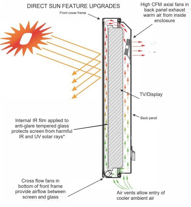
\*To maintain the effectiveness of the anti-glare glass and maintain picture quality, the screen must be mounted so that the front of it is between 0.75 in. and 1.20 in. from the glass.
