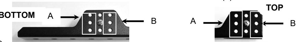
To adjust TV slightly **DOWN** in the enclosure, move roller one row toward the top of the bracket on both ends of each bracket. See (B)
